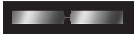
Fig. 2 Silver link semiconductor fuse.
